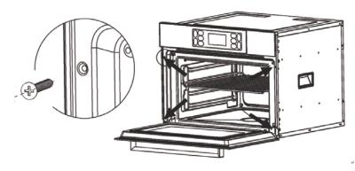
First, lift up the appliance and put it inside the preserved area in the cabinet. (Pay attention to the power plug location, such to connect the electricity after installation). Open the oven door, tighten the 4 screws supplied to the 4 holes of the inner door frame. Make sure that the appliance is fixed in place before connect to the electricity.
